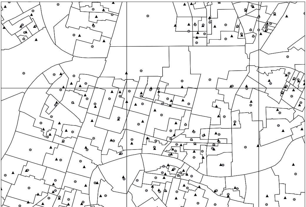
Figure 2 Aggregation of spatial districts by means of their centroids (circles) or centroids of populated buildings (triangles) into 1 \text{ km} \times 1 \text{ km} grid
