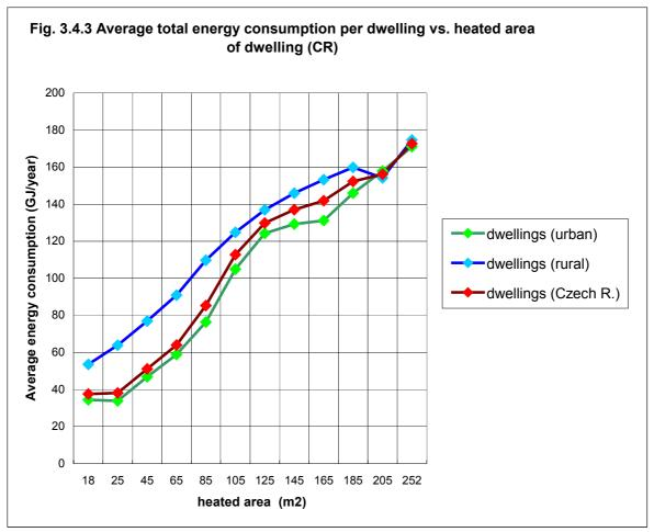
This figure (graph 3.4.3) shows energy consumption vs. heated floor area relationship. About 80% of energy in dwellings is consumed by space heating that is closely related to the size of heated floor area. The shape of the relationship is also affected by the sample size and the number of dwellings in urban localities or rural localities where this relationship is of rather different character, as it is evident from curves course.
