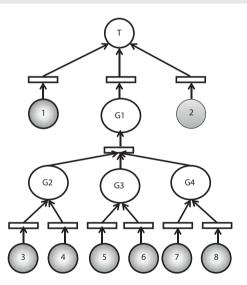
Note: T: top event, G: gate (fundamental operators AND, OR), a place with token: . Source: Own construction
