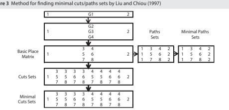
Figure 3 Method for finding minimal cuts/paths sets by Liu and Chiou (1997)
