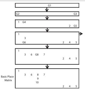
Figure 8 Basic Place Matrix of the 1<sup>st</sup> motor in "three-motor" system for finding minimal cut/path sets by method Liu and Chiou (1997)
